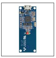
The ACM1252U-Z2 is an NFC reader module developed based on the 13.56 MHz contactless technology. This NFC Reader Module supports all three NFC modes: card reader/writer, card emulation, and peer-to-peer communication.
